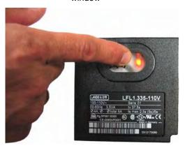
Indicator dial provides symbolic information about the program sequence, the type of fault, and the point in the sequence where the fault occurred.
