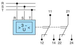
L1 - L2 - L3 : 3-phase network being monitored 11 - 12 - 14 : Output relay (R1) lower threshold 21 - 22 - 24 : Output relay (R2) upper threshold
