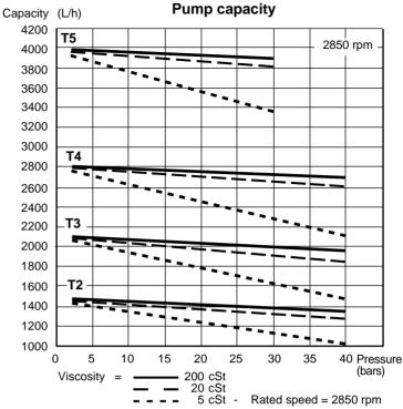
Data shown are for new pumps, with no allowance for wear.
